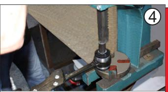
Apply grease to the I.D. & O.D. of 03P03474 & 03P03575 and all metal parts that will contact the new polyurethane bushings. Press in the new bushings and sleeve into the shell in the order shown above. Install the control arm back into the vehicle and torque all fasteners to factory specs.
